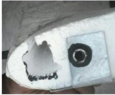
Figure 6 Cavity to accommodate the synthetic jet mechanism
