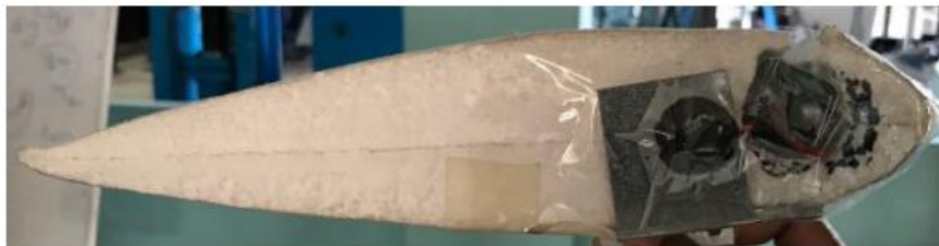
Figure 7 Synthetic Jet mechanism inside
